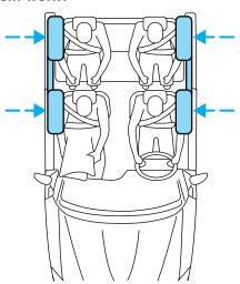
seat. The air curtain was designed to inflate between the side window area and occupant to further enhance the head protection provided to occupants in side impact collisions. The seat-mounted side airbag was designed to inflate between the door panel and occupant to further enhance the protection provided occupants in side impact collisions.
